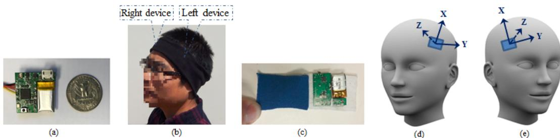
Fig. 3. Wearable device. (a) Hardware platform Zhao et al. (2017); (b) Device deployment; (c) Device covered by two polyester tapes; (d) Sensor orientations of the left device; (e) Sensor orientations of the right device
