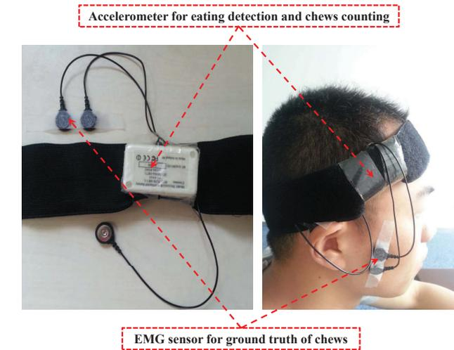
Fig. 1. Data collection device and deployment
