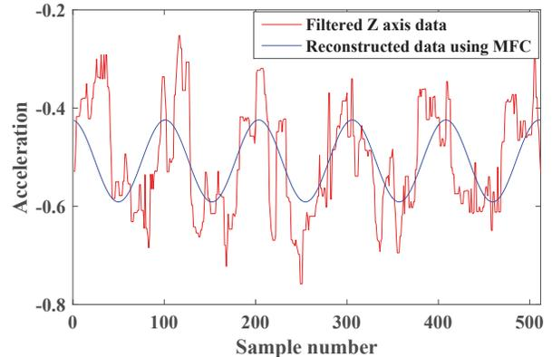
Fig. 6. Noisy acceleration data and reconstructed data using MFC
