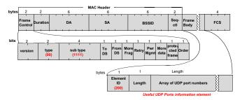
Fig. 3. Frame structure of UDP port message
