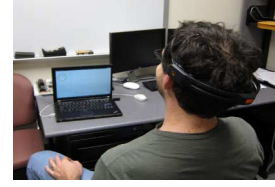
Fig. 2. Neuroheadset working with a laptop as base station.
