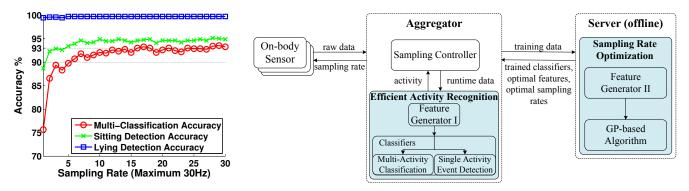
Figure 1. Accuracies of sitting and lying down event Figure 2. AdaSense architecture. **Note:** The sampling rate optimization and classifier training are detections as well as multi-activity classification vs performed on the server offine. No communication occurs between aggregator and server in runtime. Sampling rate.
