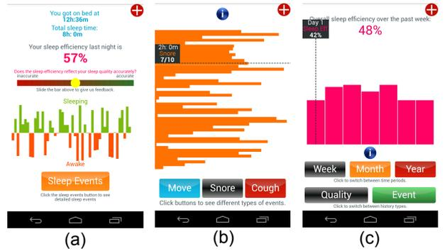
**Figure 17: The user interface of iSleep. (a) The screen showing sleep efficiency and sleep states over night. (b) The screen showing the sleep events detected overnight and the normalized loudness of each event. (c) The screen showing the history of sleep efficiencies and events.**
